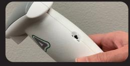
Move the switch, located on the back of the PDS to the "ON" position.
